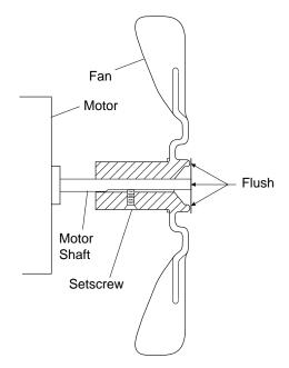
Figure 7 - Fan Cross Section
